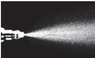
Injector spray pattern after P.i. treatment.
